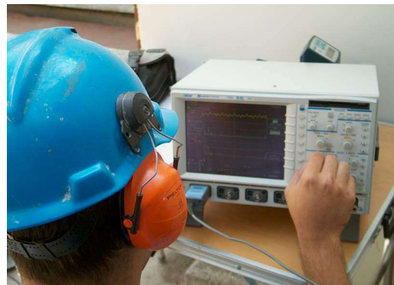
Measures of the shaft tension
